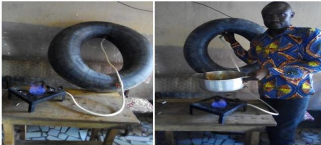
Photo 11: Biogas combustion test
